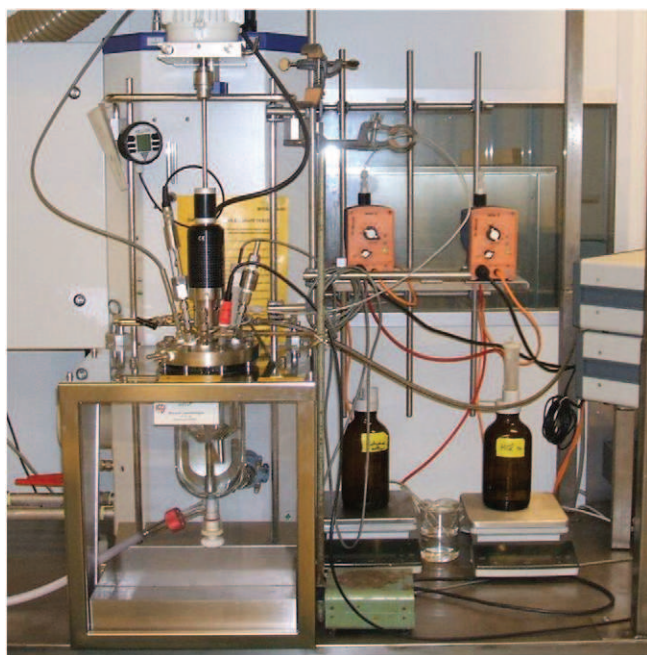
Fig. 1. RC1 unit: stirred batch reactor equipped with two feeding pumps and temperature and pH sensors.
