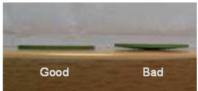
Fig. 10. Optical photographs of two anode discs after the 1400^\circ\text{C} sintering. The right one is not flat enough in order to characterize the gas-tightness of the top electrolyte in the lab-scale permeation cell.
