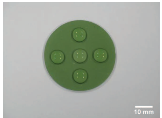
Fig. 7. Water drops deposited on sample E after a co-firing treatment at 1400 \text{ }^\circ\text{C} . The YSZ coating was deposited by the spin-coating technique, using a rotational rate of 3000 \text{ rpm} and a ratio Rm equal to 0.25 (sample #E). The water drops were not drained after 5 min.
