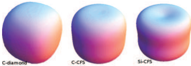
FIG. 1. (Color online) Three-dimensional representations of elastic constants of carbon (C) diamond, C-CFS, and Si-CFS.
