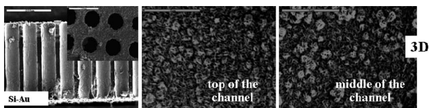
Fig. 19 CuS electrodeposited on perforated (3D) silicon substrates. The scale bars indicate 200 \mu\text{m} on the left most image and 5 \mu\text{m} on the two right most images. The left most image gives a global representation of the deposition over the pores. The two right-most images give an idea of the microscopic differences in the quality of the deposit at the top and in the middle of the channel, indicating a conformal deposition. Reprinted with permission from ref. 36.
