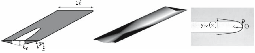
Fig. 2 (a) Sketch of flat straight linear channel with h_0 = 1 mm, \ell = 25 mm. (b) Perspective view of a linear constricted channel. (c) Top view showing the comparison between the experimental bubble invading channel depicted in Fig. 2a with gray line and Fig. 2b in black line
