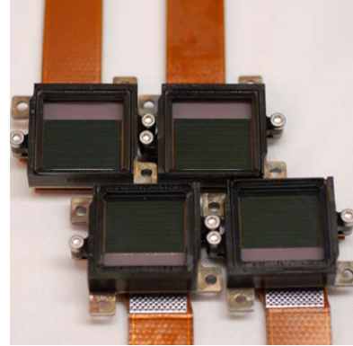
Figure 17 : Four EM models in staggered configuration
