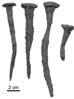
Fig. 1. Nails from the Uxellodunum site from which the PM98 steel samples have been selected (photo courtesy of Renoux and Dabosi).
