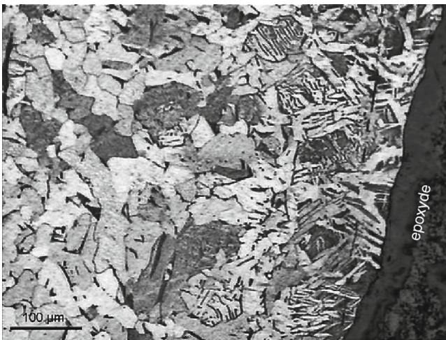
Fig. 2. Optical micrograph of the PM98 nail. On the left, inner part of the nails with ferritic grains and carbides precipitated at the grains boundaries; in the center, pearlitic colonies; near the surface, Widmanstätten structure. The dark layer on the right part of the micrograph is the epoxyde used for sample preparation.
