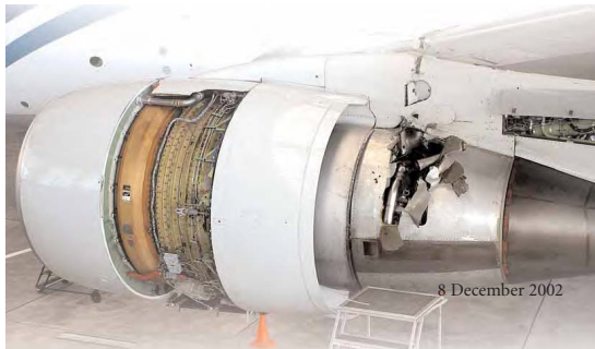
(a) Uncontained engine failure Boeing 767 (Australian Airline).
