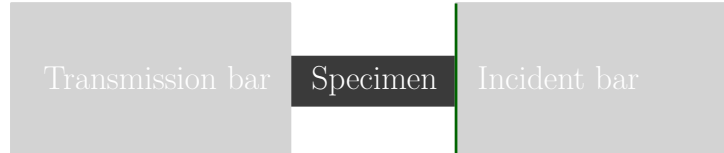
Figure 3.12: Schematic representation of incident bar and specimen interface.
