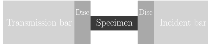
Figure 3.15: Schematic representation of incident/transmission bar and discs.
