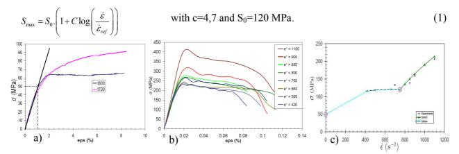
**Figure 1. a)** Quasi-static tension of T700/M21S and T800/M21S [±45°]<sub>2s</sub>; **b)** Dynamic compression of T800/M21S [±45°]<sub>3s</sub>; **c)** Strain rate effects on T800/M21S [±45°]<sub>2s</sub> lamina strength.
