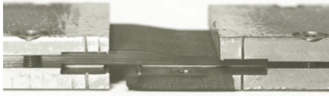
Fig. 4 Specimen clamped in the anti-buckling device
