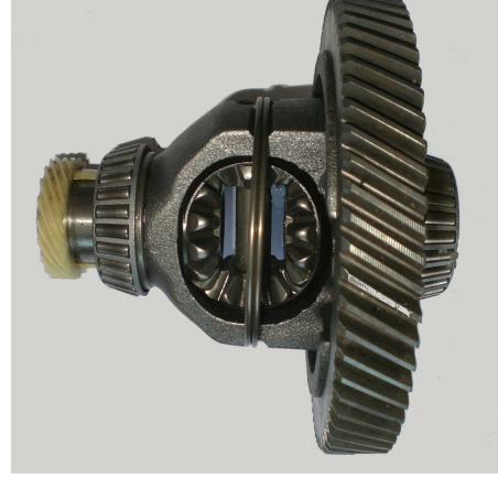
Figure 4: Picture of the car differential
