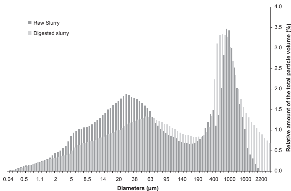
Fig. 2. Distribution of the relative volumes of the various size classes of particles in raw and digested slurry.
