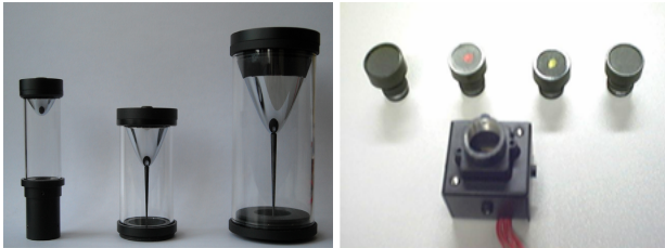
Fig. 5. The three hyperbolic mirrors and one small camera.
