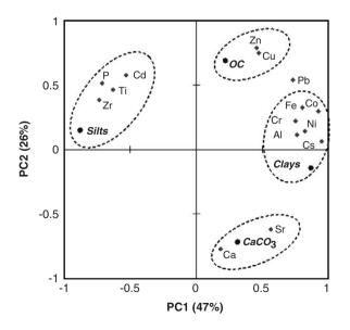
Fig. 10. Principal component analysis performed on the entire heavy metal dataset, including sediment properties (i.e. clay, silt, OC and carbonate contents, n = 47).
