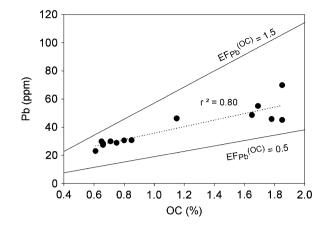
Fig. 12. Relationship between OC contents and total Pb contents in the surficial prodeltaic sediments (n = 14). The two lines correspond to metal enrichment factor of 1.5 and 0.5, respectively, showing that no significant enrichment is found when EF is normalized to OC. Similar results are found with Cu and Zn.
