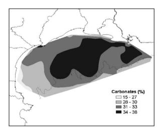
Fig. 4. Spatial distribution of carbonate contents (%) in surficial sediments of the Gulf of Lions ( $<63 \,\mu m$ ).
