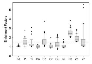
Fig. 8. Enrichment factors of investigated elements in the less than  $63 \,\mu\text{m}$  surficial sediment fraction. Major and trace elements were normalized using the local backgrounds as natural references (see text). The dashed line represents the natural variability threshold (EF = 1.5).
