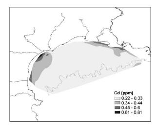
Fig. 7. Spatial distribution of Cd contents in the less than  $63\,\mu m$  surficial sediment fraction.
