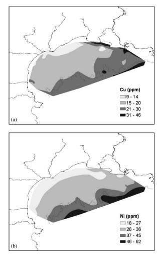
Fig. 6. Spatial distribution of Cu and Ni contents in the less than  $63 \,\mu m$  surficial sediment fraction. Notice that the higher enrichment of Cu off the river mouths is likely influenced by its affinity with organic carbon.
