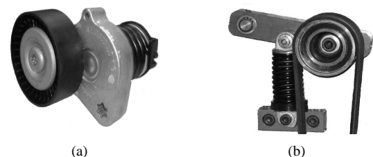
Fig. 1. Tensioner types: dry friction( a) and hydraulic (b).
