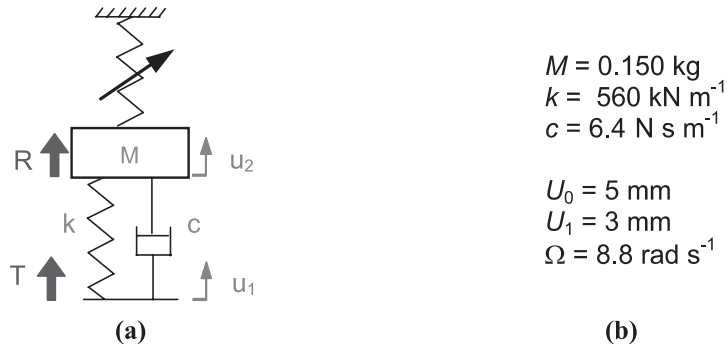
Figure 7. Schematic view (a) and photograph (b) of the test rig 2 devoted to the validation test.
