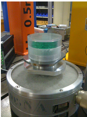
Figure 1: First experimental set-up. Transparent box filled of particles, embedded on a electrodynamic shaker
