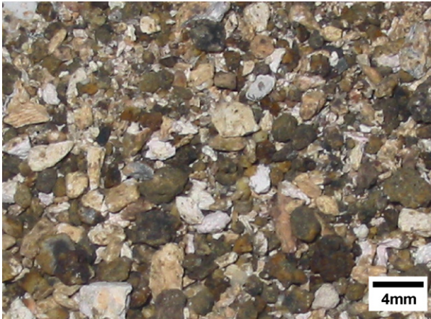
Fig. 6. Industrial meat and bone meal bottom ash (MBM-BA).
