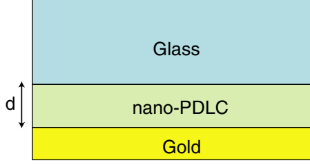
Fig. 7. Three-layer structure retained for the calculation of the guided modes. The parameters are the same as in Fig. 5.
