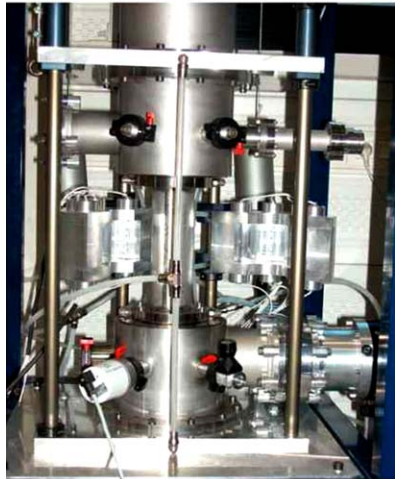
Fig. 2. View of the central part of the tribometer showing the test chamber surrounded by the radiative furnace and the two satellite-crowns containing the driving and loading shafts and the water jackets.
