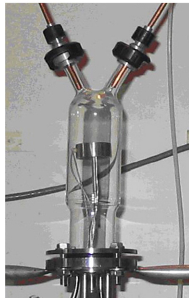
Fig. 3. Deposition chamber (heating resistor inside the sample's support).
