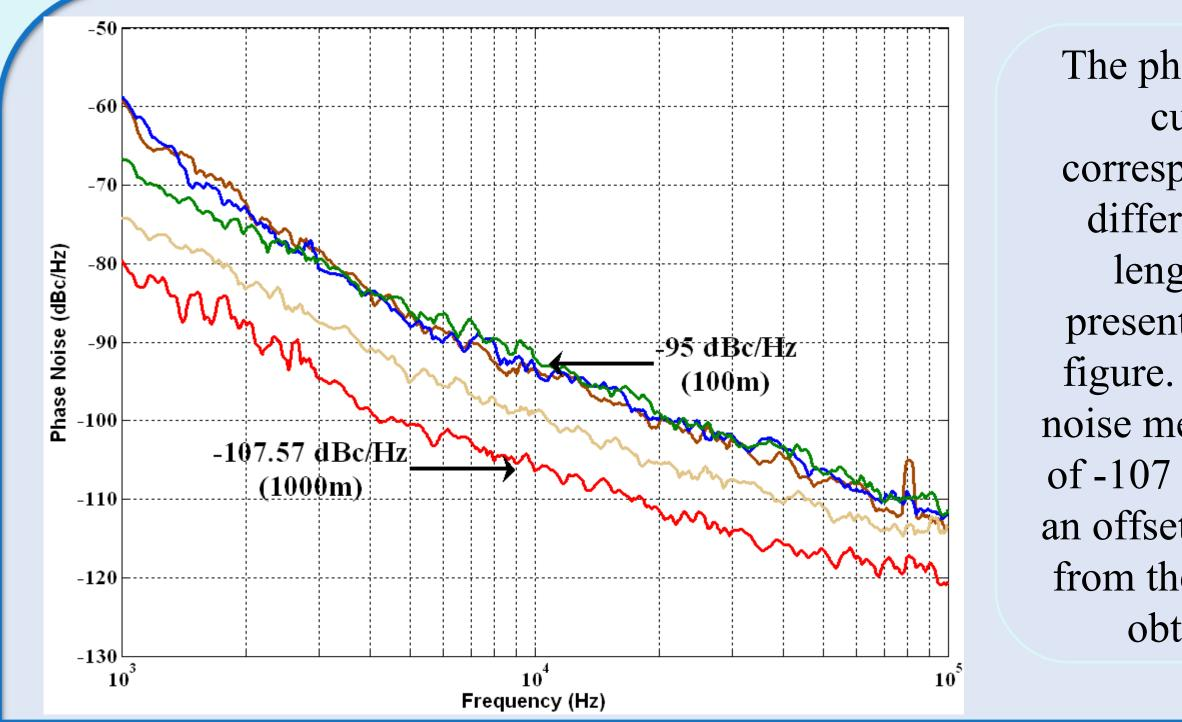
The phase-noise curves corresponding to different fiber lengths are presented in this figure. A phasenoise measurement of -107 dBc/Hz at an offset of 10 kHz from the carrier is obtained.
