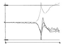
FIGURE 2: angle of attack i(t) (solid) and wind profile w(t) (dashed).
