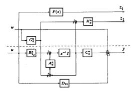
FIGURE 1:  $P_f(z)$ : setup for the final  $H_{\infty}$  synthesis.
