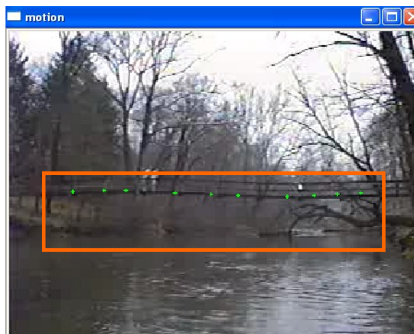
Figure 1: Example of motion estimation, using an adaptation of lkdemo algorithm. The 10 initialization points are in green full circle and the zone under study is in orange.
