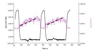
Alternating stepped shear stress below and beyond the threshold (figure above) shows that the fluid can partly recover its structure. This explains why a continuous air injection leads to a more deflocculated sludge than an intermittent one. Moreover, this displays that pauses during the aeration process are of greatest interest and give keys to propose efficient aeration.
