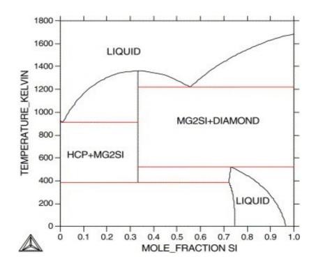
The figure shows an attempt to reproduce the stable phase diagram by just refitting the liquid description with two Redlich–Kister excess parameters with an exponential temperature dependence according to that model:
