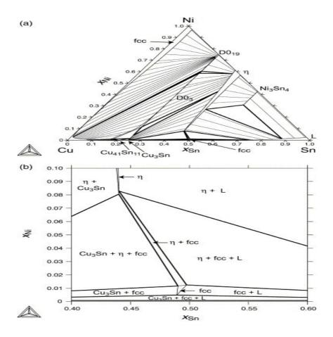
Fig. 7. Calculated isothermal section of the Cu–Sn–Ni phase diagram at 773 K. (a) Entire composition range, (b) detail showing the artificial appearance of the fcc phase in Sn-rich alloys near the Cu–Sn binary edge.
