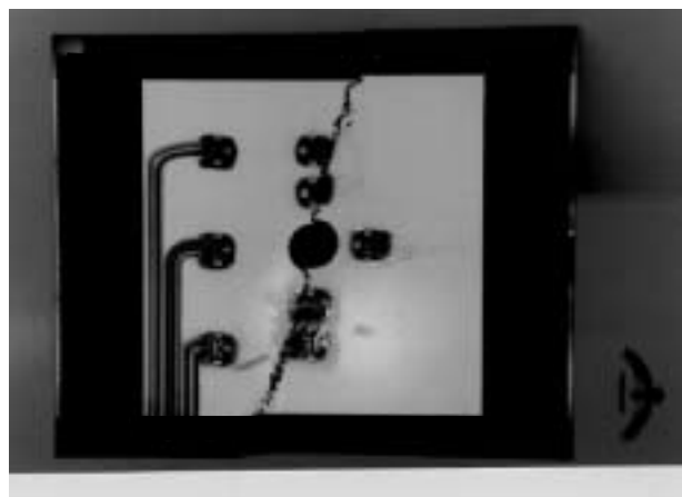
Fig. 25—Failure pattern under combined load of an impacted specimen
