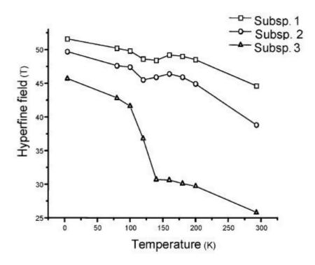
Figure 4 Temperature dependence of the hyperfine field for the three subspectra (subsp. 1 and 2 for octahedral Fe; subsp. 3 for tetrahedral Fe).
