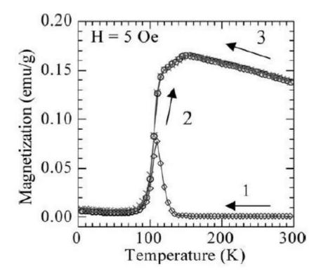
Figure 1 Temperature dependence of the magnetization in 5 Oe on first-cooling (1) and warming (2) and second-cooling (3).
