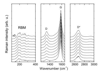
FIG. 2: Transformed DWCNT filled by PbI2 after a pressure of 25 GPa acquired in the hole gasket. The spectra are sorted by D band intensity.
