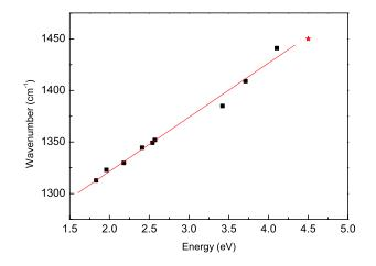
FIG. 3: Frequency of the D band in air as a function of the exciting wavelength. The star corresponds to the value deduced from overtones.
