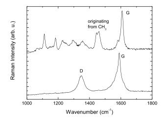
FIG. 4: Two typical spectra obtained on an heterogeneous composite (0.4 % in weight of CNT and 0.4 % in weight of palmitic acid).
