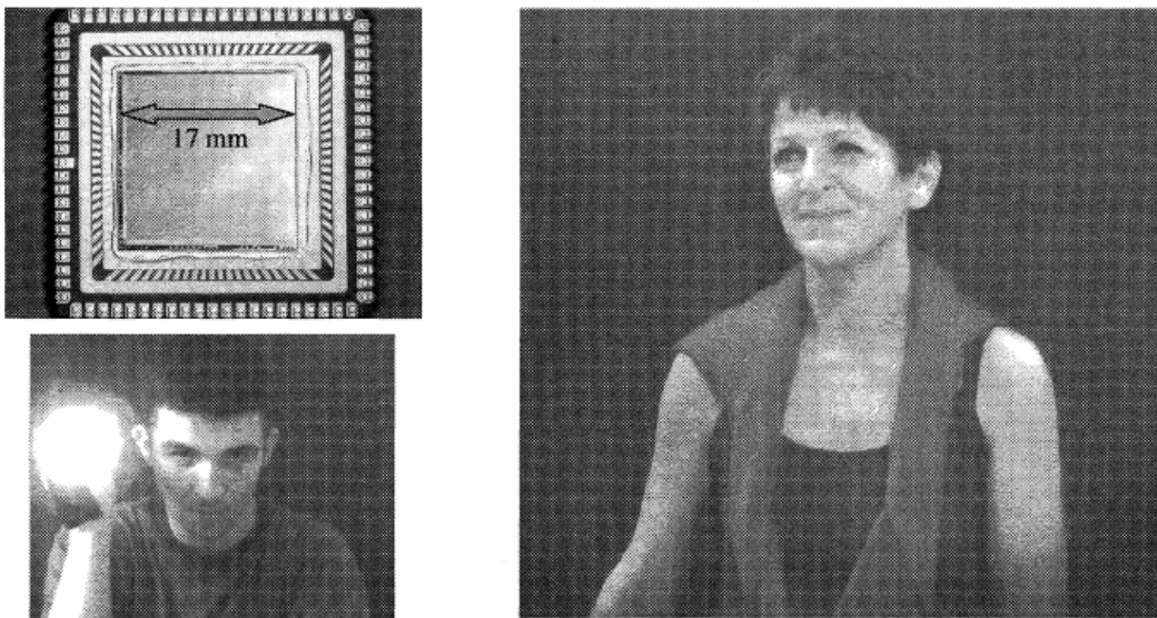
Figure 3-a (left-top): view of the CMOS512 image sensor within its package. Figure 3-b (right): rough image (only FPN corrected) obtained using the CMOS512 device operated at 4 Mpixels/s. Figure 3-c (left-bottom): demonstration of the anti-blooming capability of the device
