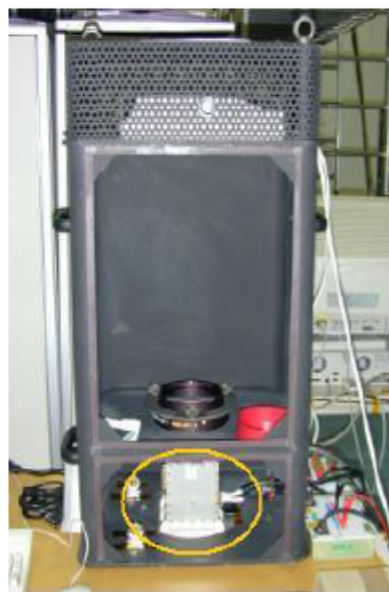
Fig. 5: Star tracker camera under functional test
