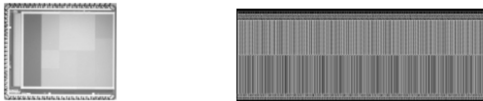
Figure 3: (a) left: test vehicle built through a CNES R&T contract in order to improve pixel performances using standard CMOS technologies; (b) right: layout of a linear array with CTIA injection stages devoted to pushbroom Earth observation
