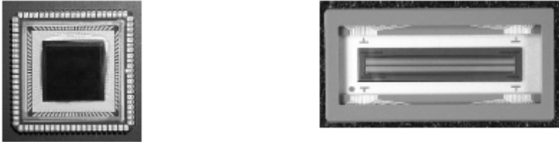
Figures 5: 1k x 1k 2D array (left) and 3k linear array (right) in their corresponding packages
