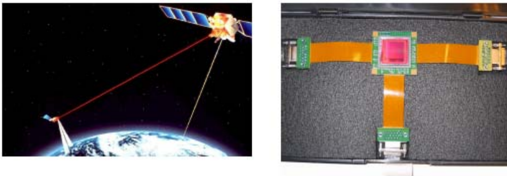
Fig. 5-a: left: SPOT 4 images transmission down to ground via optical link and ARTEMIS relay overcomes intermittent radio electrical visibility from its ground network; Fig. 5-b: right: CIS acquisition and tracking sensor developed by EADS Astrium and Supaéro/CIMI
