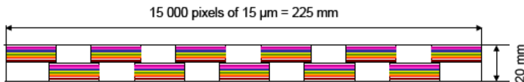
Fig. 6: thanks to CIS architecture flexibility and low power dissipation, high performances multispectral CMOS linear arrays can be manufactured. Butting several of them would lead to large superspectral focal planes
