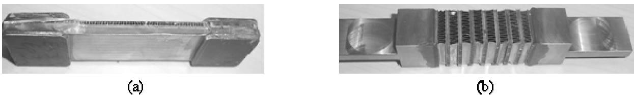
Fig. 2 . Tensile test samples along (a) z-axis (b) y-axis
