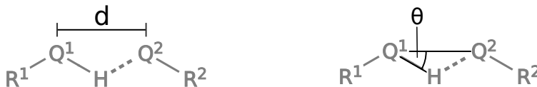
Figure 28: Geometrical description of a hydrogen bond by the distance d between the electronegative centers and the angle \theta between the acceptor ( Q^2 ), the donor ( Q^1 ) and the hydrogen.
