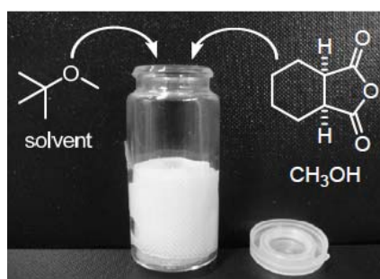
Figure 4-4. Reaction set-up using the textile-based catalyst shown as the white material contained in the vial.
