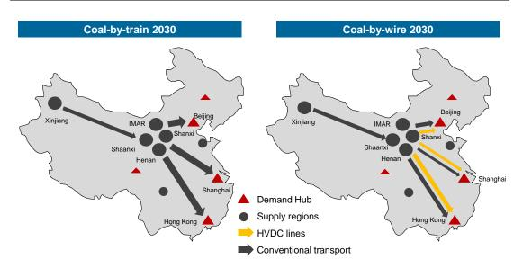
FIGURE 5.2: Topology of the scenario setup for China
