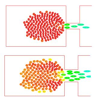
Figure 5.7: Screenshot of a simulation with strategy 3. Top: Width of the bottleneck  $w=1.2\,\mathrm{m}$ . Bottom: Width of the bottleneck  $w=2.5\,\mathrm{m}$
