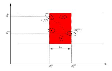
Figure B.1: Pedestrian i enters the measurement area (red) at  $t_i^{\text{in}}$  in  $(x_i^{\text{in}}, y_i^{\text{in}})$  and leaves it at  $t_i^{\text{out}}$  in  $(x_i^{\text{out}}, y_i^{\text{out}})$ . The direction of motion is from left to right.
