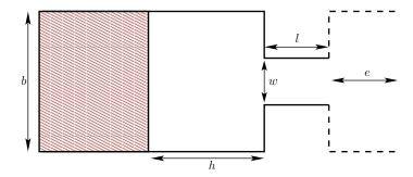
Figure 5.1: Scenario set-up. Pedestrians move from a holding area (shaded area) through the bottleneck ( $l=2.8\,\mathrm{m},\ h=4.5\,\mathrm{m},\ b=4\,\mathrm{m}$  and w variable).  $e=2\,\mathrm{m}$  is the length of the extra space adjacent to the bottleneck.
