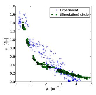
Figure 6.5: Density-velocity relation with *circles* in a corridor of dimensions  $25 \times 1 \text{ m}^2$  in comparison with experimental data obtained in the HERMES-project [39]. In these simulations b is set to be equal to a.
