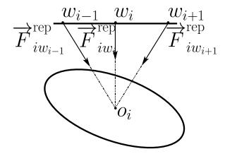
Figure 3.3: Each wall is modeled as three static point masses acting on pedestrians.
