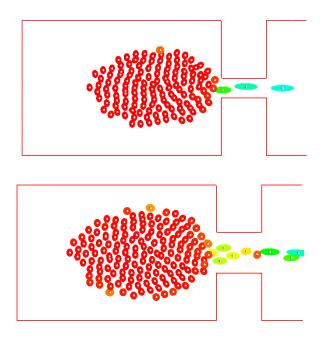
Figure 5.3: Screenshot of a simulation with strategy 1. Top: Width of the bottleneck  $w=1.2\,\mathrm{m}$ . Bottom: Width of the bottleneck  $w=2.5\,\mathrm{m}$
