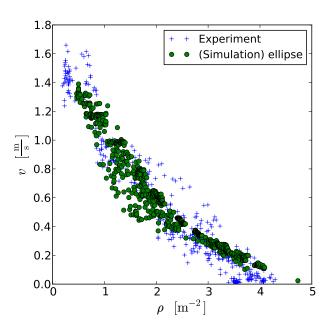
Figure 6.4: Density-velocity relation with *ellipses* in a corridor of dimensions  $25 \times 1 \text{ m}^2$  in comparison with experimental data obtained in the HERMES-project [39].
