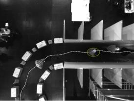
Figure 4.1: Off-line trajectory detection with PeTrack [4]. Left: The trajectory of the detected pedestrian shows strong swaying. Right: The faster pedestrians move, the smoother and weaker is the swaying of their trajectories.
