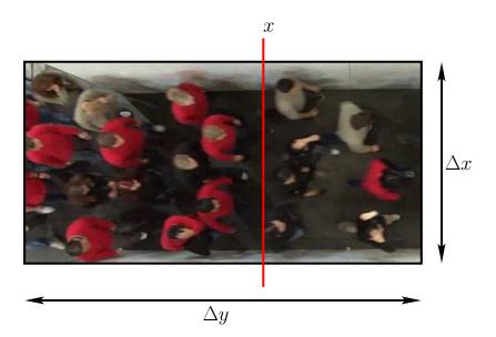
Figure 1.3: Calculating the average of the quantities v, J and  $\rho$  by averaging over time or over space; Average of the velocity and flow of pedestrians crossing the line x during a measurement period  $\Delta t$  and the average over the space  $(\Delta x \times \Delta y)$  of the velocity and the density. The missing observable cat be calculated using the relation  $J \propto v\rho$ .
