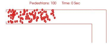
Figure 5.13: Simulation set-up: 100 pedestrians move around the corner with help of guiding lines. Corridor-width is 3 m and its length is 18 m.
