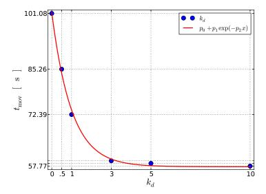
Figure 5.20: Movement time for a simulation with N=100 pedestrians around a corner for different values of  $k_d$ . The parameters  $p_i$  of the optimal fit (red curve) were calculated with the Levenberg-Marquandt algorithm [70].
