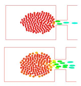
Figure 5.9: Screenshot of a simulation with strategy 4. Top: Width of the bottleneck  $w=1.2\,\mathrm{m}$ . Bottom: Width of the bottleneck  $w=2.5\,\mathrm{m}$ .
