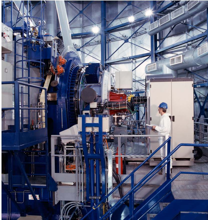
Fig. 1.4.: NAOS/CONICA at the Nasmyth focus of VLT UT 4, Yepun. The red cylinder is the camera system CONICA. Image courtesy:ESO.
