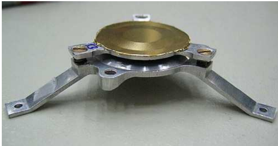
Figure 3.2: A gold stopper foil is mounted and stretched on the aluminum cone.
