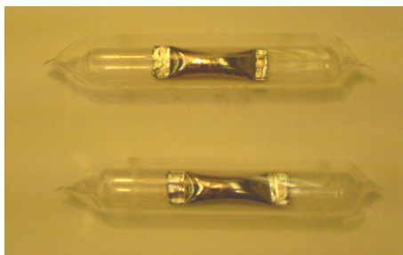
Figure 2.3.: Tantalum containers sealed in silica ampoules.
