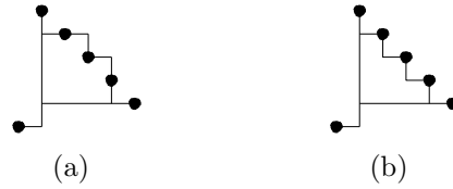
Figure 6.13: (a) The set MN before calling Procedure 12 MAKE ENVELOPE. (b) The set MN after calling Procedure 12 MAKE ENVELOPE.
