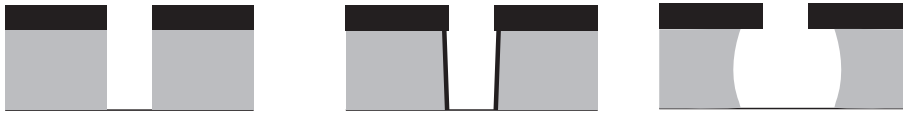
Fig. 3.24: Schematic illustration of the difference between fully anisotropic (left), isotropic with side-wall passivation (middle) and fully isotropic (right) etch. The resist mask is black and the etched material grey.
