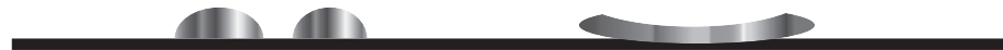
Fig. 3.7: Schematic representation of a thin compressive film (left) and a thin tensile film (right). A compressive film tends to build discontinuities. A tensile film tends to peel off the substrate. The gas pressure in the sputtering chamber can be varied to control film stress.
