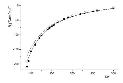
Figure 4.14: Second virial coefficient of fluorine. —: calculated by Eq. 3.5 and - - -: calculated by Eq. 3.6 (this work),  $\circ$ : calculated with Deiters equation of state (D1) [18],  $\bullet$ : experimental data [17, 28].
