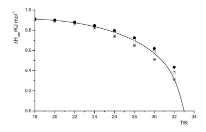
Figure 4.18: Vaporization enthalpy of hydrogen. Symbols: —, experimental data [76, 66];  $\circ$ , modified Benedict-Webb-Rubin equation of state [139];  $\bullet$ , \*: *ab initio* pair potentials Eq. 3.3 and Eq. 3.4.
