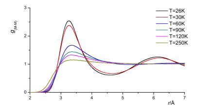
Figure 9.4: Temperature dependence of  $g_{\rm M-M}$  for hydrogen at P = 1.0 MPa from GEMC NPT simulation using the pair potential Eq. 3.3.
