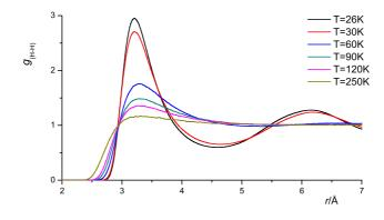
Figure 9.2: Temperature dependence of  $g_{\rm H-H}$  for hydrogen at P = 1.0 MPa from GEMC NPT simulation using the pair potential Eq. 3.3.
