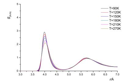
Figure 10.15: Temperature dependence of  $g_{\rm N-N}$  for fluorine at P = 10.0 MPa from GEMC NPT simulation using the pair potential Eq. 3.6.
