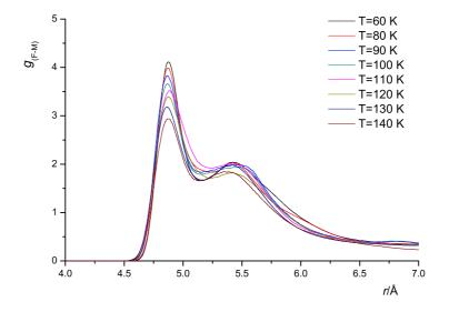
Figure 10.25: Temperature dependence of  $g_{\rm F-M}$  for the liquid phase fluorine from GEMC NVT simulation using pair potential Eq. 3.6.
