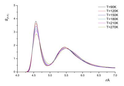
Figure 10.14: Temperature dependence of  $g_{\rm F-F}$  for fluorine at P = 10.0 MPa from GEMC NPT simulation using the pair potential Eq. 3.6.
