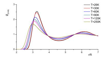
Figure 9.17: Temperature dependence of  $g_{\rm H-M}$  for hydrogen at P = 5.0 MPa from GEMC NPT simulation using the pair potential Eq. 3.4.
