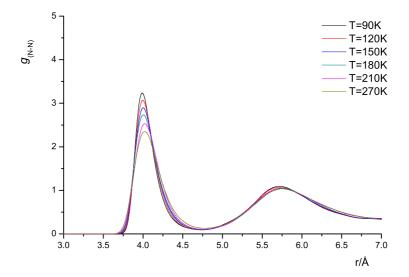
Figure 10.11: Temperature dependence of  $g_{\rm N-N}$  for fluorine at P = 1.0 MPa from GEMC NPT simulation using the pair potential Eq. 3.6.
