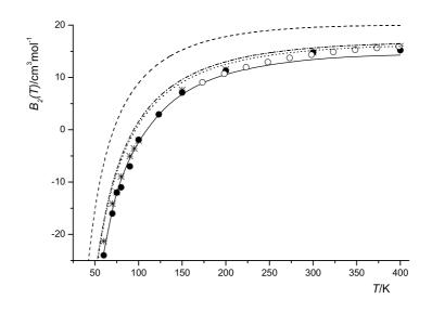
Figure 4.8: Second virial coefficients  $B_{cl}^0$  of hydrogen using the pair potential Eq. 3.3 resulting from CCSD(T) level of theory; - - -: aug-cc-pVDZ; - - - -: aug-cc-pVTZ; ...: aug-cc-pVQZ; —: aug-cc-pV23Z; •: experimental data [28, 66]; •: Lennard-Jones potential by Wang [132]; \*: spherical harmonic potential by Etters and Diep [32, 25, 26].
