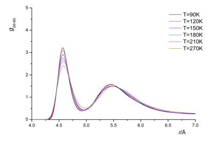
Figure 10.16: Temperature dependence of  $g_{\rm M-M}$  for fluorine at P = 10.0 MPa from GEMC NPT simulation using the pair potential Eq. 3.6.
