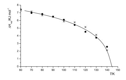
Figure 4.21: Vaporization enthalpy of fluorine. Symbols: —, experimental data  $[17]; \bullet, *: ab initio$  pair potentials Eq. 3.5 and Eq. 3.6.
