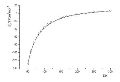
Figure 4.15: Cross second virial coefficient of the hydrogen-fluorine system. —: calculated from Eq. 3.5 and - - -: calculated from Eq. 3.6 (this work);  $\circ$ : calculated from empirical correlation [30, 31].
