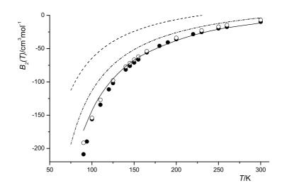
Figure 4.11: Second virial coefficients  $B_{cl}^0$  of fluorine using the pair potential Eq. 3.6 resulting from CCSD(T) level of theory; for an explanation of the symbols see Fig. 4.10 and text.
