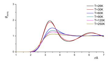
Figure 9.3: Temperature dependence of  $g_{\rm N-N}$  for hydrogen at P = 1.0 MPa from GEMC NPT simulation using the pair potential Eq. 3.3.
