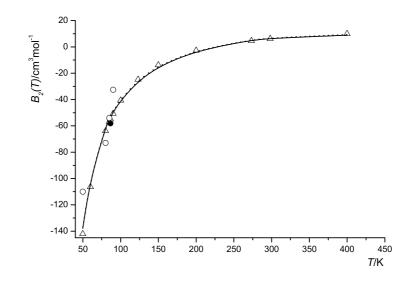
Figure 4.13: Cross second virial coefficient of the hydrogen-oxygen system. —: *ab initio* prediction (this work) based on Eq.  $(3.3), \cdots$ : prediction based on Eq.  $(3.4), \Delta$ : calculated from empirical correlation [31, 30], •: interpolation from neon mixtures (see section 4.2.2); other symbols: experimental data (see Table 8.3).
