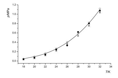
Figure 4.17: Vapor pressure of hydrogen. Symbols: —, experimental data [76, 66];  $\circ$ , modified Benedict-Webb-Rubin equation of state [139];  $\bullet$ , and \*: ab initio pair potentials Eq. 3.3 and Eq. 3.4.
