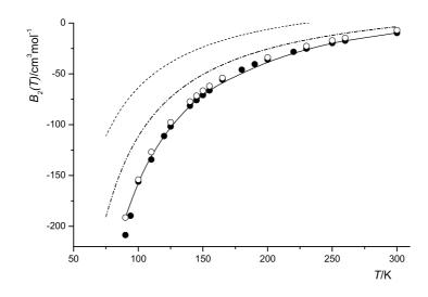
Figure 4.10: Second virial coefficients  $B_{cl}^0$  of fluorine using the pair potential Eq. 3.5 resulting from CCSD(T) level of theory; - - -: aug-cc-pVDZ; - - -: aug-cc-pVZZ; --: aug-cc-pV23Z; •: experimental data [17, 28]; o: calculated with Deiters equation of state (D1) [18].
