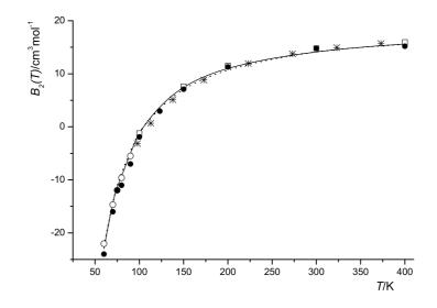
Figure 4.12: Second virial coefficients of hydrogen are calculated using the pair potentials (this work): —: pair potential Eq. 3.3;  $\cdots$ : pair potential Eq. 3.4; •: experimental data [28, 66];  $\circ$ : path integral, and  $\Box$ : semi-classical method (Diep [25, 26]); \*: Lennard-Jones 6-12 potential [79].
