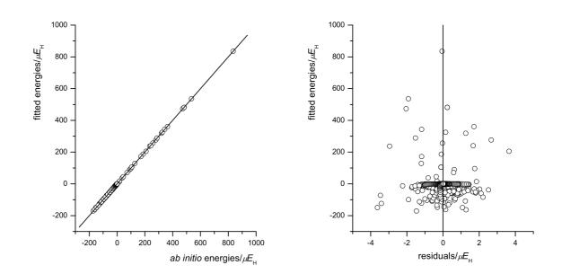
Figure 4.6: Quality of the 5-site *ab initio* analytical potential fit Eq. 3.3 for hydrogen at the theoretical level CCSD(T)/aug-cc-pV23Z.
