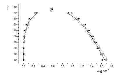
Figure 4.19: Vapor-liquid coexistence diagram of fluorine. Symbols: —, experimental data [17];  $\circ$ , Lennard-Jones potential [90];  $\cdots$ , Deiters equation of state (D1 EOS) [18];  $\bullet$ , \*: *ab initio* pair potentials Eq. 3.5 and Eq. 3.6.
