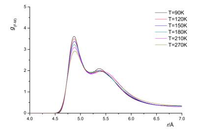
Figure 10.17: Temperature dependence of  $g_{\rm F-M}$  for fluorine at P = 10.0 MPa from GEMC NPT simulation using the pair potential Eq. 3.6.
