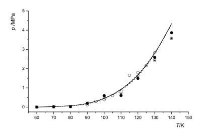
Figure 4.20: Vapor pressure of fluorine. Symbols: —, experimental data [17];  $\circ$ , Lennard-Jones potential [90];  $\cdots$ , Deiters equation of state (D1 EOS) [18];  $\bullet$ , \*: *ab initio* pair potentials Eq. 3.5 and Eq. 3.6.
