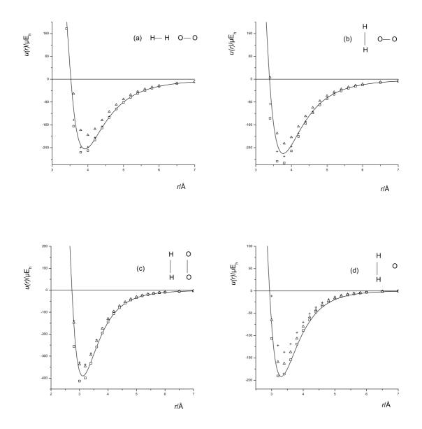
Figure 6.2: Intermolecular potentials of  $H_2$ - $O_2$ ; for an explanation see Fig. 6.1.
