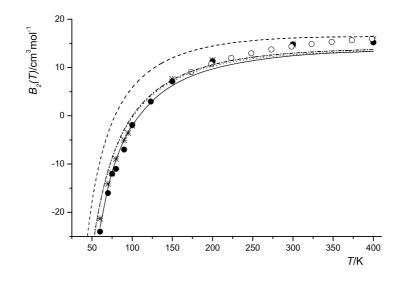
Figure 4.9: Second virial coefficients  $B_{cl}^0$  of hydrogen using the pair potential Eq. 3.4 resulting from CCSD(T) level of theory; for an explanation of the symbols see Fig. 4.8 and text.
