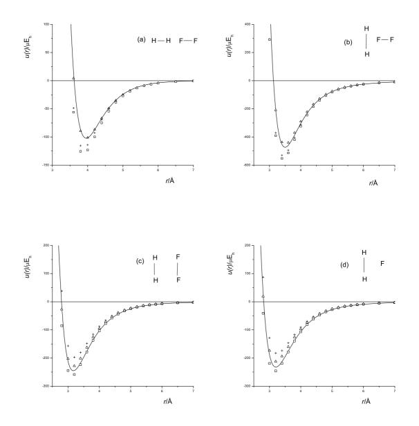
Figure 6.4: Intermolecular potentials of  $H_2$ - $F_2$ ; for an explanation see Fig. 6.1.
