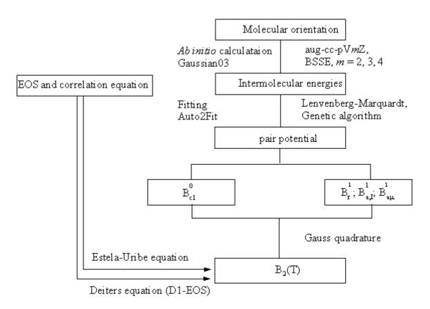
Figure 3.3: The block diagram for calculating the virial coefficients  $B_2$ .
