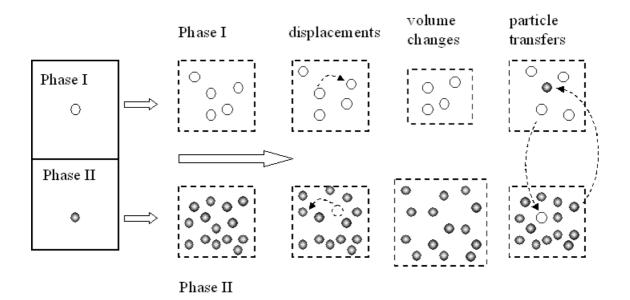
Figure 2.1: Scheme of the Gibbs ensemble technique [93]. Dotted lines indicate periodic boundary conditions.
