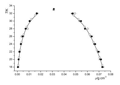
Figure 4.16: Vapor-liquid coexistence diagram of hydrogen. Symbols: —, experimental data [76, 75];  $\circ$ , modified Benedict-Webb-Rubin equation of state [139];  $\diamond$ , simulated by Wang and Johnson using Silvera and Goldman (SG) potential [131]; •, \*: *ab initio* pair potentials Eq. 3.3 and Eq. 3.4.
