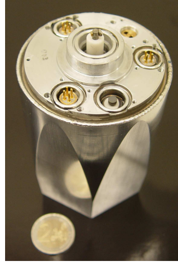
Figure 2.2: Picture of a 12-fold segmented encapsulated MINIBALL crystal.
