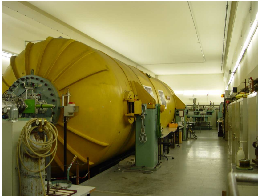
Figure 2.2: 10 MV Tandem Accelerator of the Nuclear Physics Institute (IKP) of the University of Cologne.
