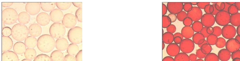
Figure 3-10: Resin beads after treatment with NF31 (left: negative test; right: positive test).
