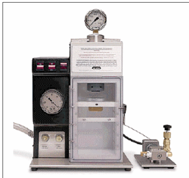
Abb. 22: Particle Delivery System Biolistic PDS-1000/He der Firma BIORAD (MPIZ-Köln).
