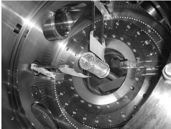
Figure 4.4: Photograph of the cryogenic target within the cyclotron trap. The pion beam enters through the Kapton window in the upper left corner. The thick plastic degrader to the right of the target and the degrader foils above and to the left decelerate the pions into the target cell.
