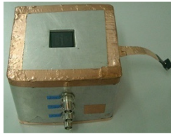
Fig. 2 Setup of the DUT enclosure
